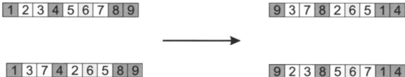
Fig. 3.17. Cycle crossover, step 1: identification of cycles
