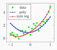
The algorithm now searches for a function  $f(x; \theta)$  and the values of  $\theta$  that minimizes the loss function  $\mathcal{L}(f; \theta; x; y)$ .
